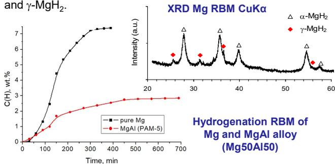
Hydrogenation RBM of Mg and MgAl alloy (Mg50Al50)
