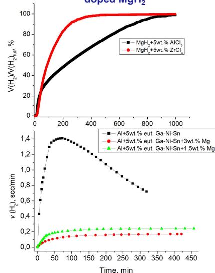
Hydrogen production rate during hydrolysis of doped Al
