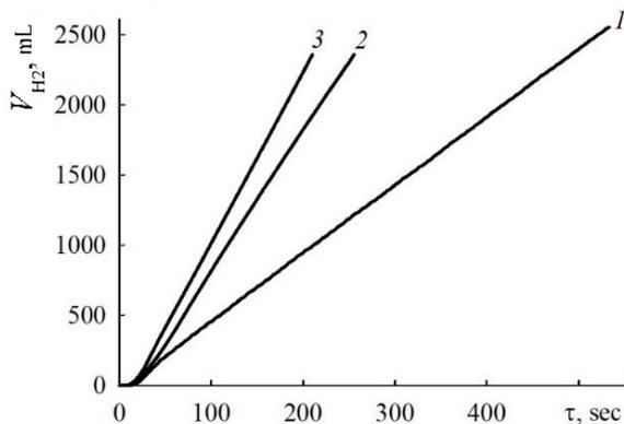
Fig. 6. Time dependencies of the volumes of the evolved hydrogen during the hydrolysis of 10 mL of the 10 %  $\text{NaBH}_4$  + 5 %  $\text{NaOH}$  solution in the 5 mL cylindrical flow reactor with  $\text{Pt}/\text{Al}_2\text{O}_3/\text{cordierite}$  catalyst at the following rates of the solution flow (mL/min): 1.1 (1), 2.4 (2) and 2.75 (3)
