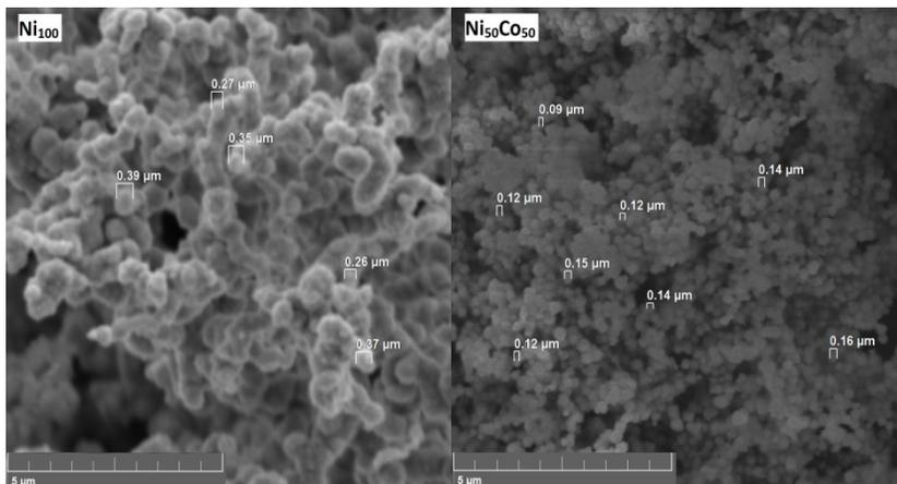
Fig. 2. SEM-images of  $\text{Ni}_{100}$  and  $\text{Ni}_{50}\text{Co}_{50}$  samples.
